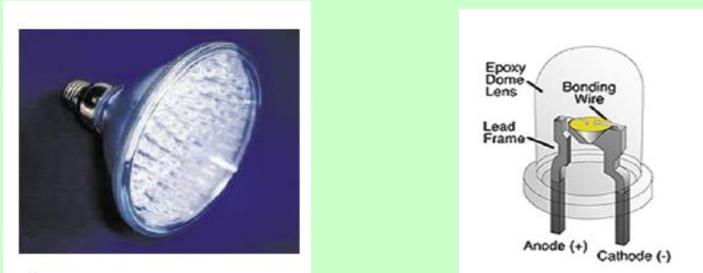
Figure 5. Picture of LED and its construction
